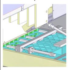
Now the pivoting plate gets into vertical position and consequently the tubes are now also in vertical position above the wholes. A pusher now presses the tubes into the tray. After the pushing hooks have indexed the tray one step ahead, this operation is repeated.
