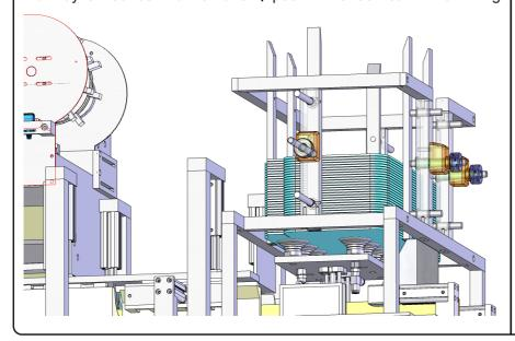
Below the holding rails is a pivoting plate, which guides the tubes from the holding rails into the wholes of the tray. If the rail at the bottoms of the tubes is removed, the tubes fall with their bottoms leading on this pivoting plate and slide in their guiding grooves to a position above the wholes of the trays.
