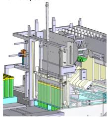
The filled trays are pneumatically pushed on a transport belt for transportation to the next packaging step.
